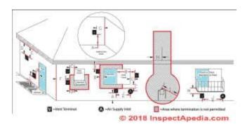
Above: Pellet stove sidewall vent terminal locations and clearance distances including from windows, doors, gas meter, roof eaves and ground surface, adapted from Harman, cited in detail below.
